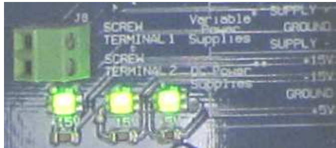
Fig. 7. Elvis Protoboard supply LEDs.
