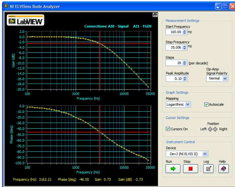
Fig 5. Bode Analyzer output and measuring the 3dB frequency using cursors.
