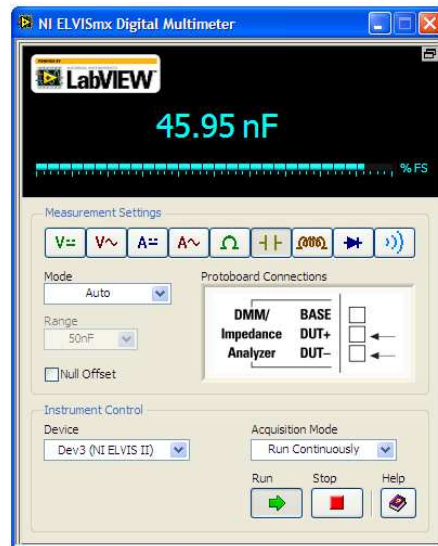
Fig. 10. Digital Multimeter SFP indicating the capacitance value.
