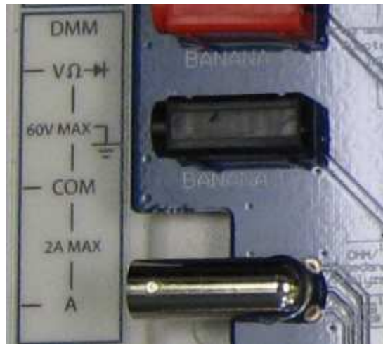
Fig. 4. DMM Ports on the Elvis Prototype Board.
