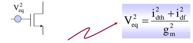
Equivalent input referred noise voltage means that all **current noise sources are accounted as drain current and represented by an "equivalent" noise voltage at transistor gate**
