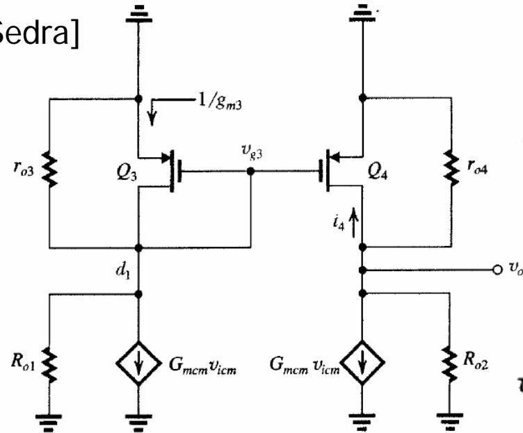
$$i_4 = -g_{m4} G_{mcm} v_{icm} \left( R_{o1} \parallel r_{o3} \parallel \frac{1}{g_{m3}} \right)$$
