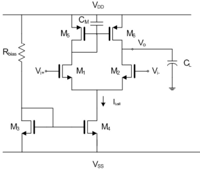
$$A_{cm} = \frac{v_o}{v_{CM}} \approx -\frac{1}{2g_{m6}r_{o4}}$$
