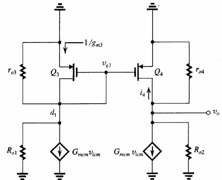
$$G_{mcm} \equiv \frac{i_o}{v_{icm}} = \frac{1}{2R_{ss}}$$
