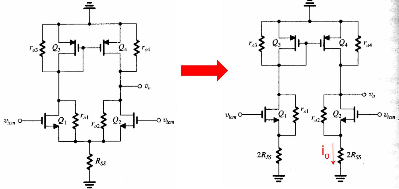
$$v_s = v_{icm} \frac{(2R_{SS} \| r_{o1})}{(2R_{SS} \| r_{o1}) + (1/g_m)} \quad i_o = \frac{v_{icm}}{2R_{SS}} \quad G_{mcm} \equiv \frac{i_o}{v_{icm}} = \frac{1}{2R_{SS}}$$
