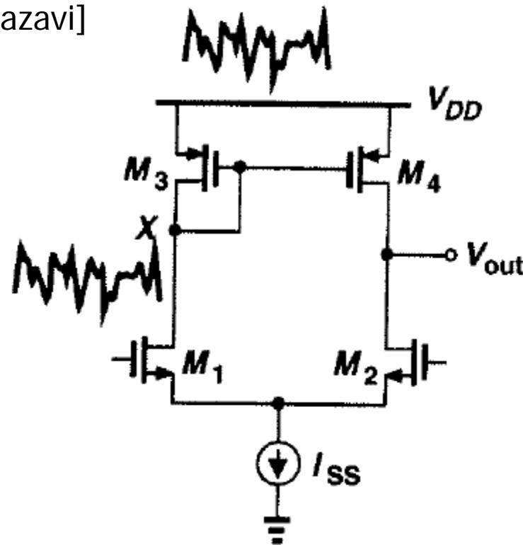
$$\text{PSRR}^+ = 20 \cdot \log_{10} \left( \left| \frac{A_{dm}}{V_o / V_{DD}} \right| \right)$$
