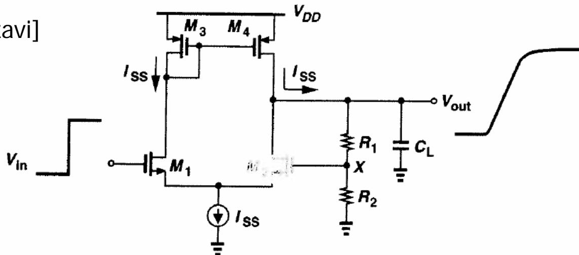
$$\text{Slew Rate} = \frac{I_{SS}}{C_L}$$
