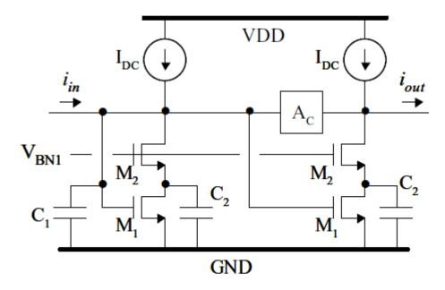
Parallel transconductance transistor MC with capacitive degeneration introduces a zero which provides frequency compensation
