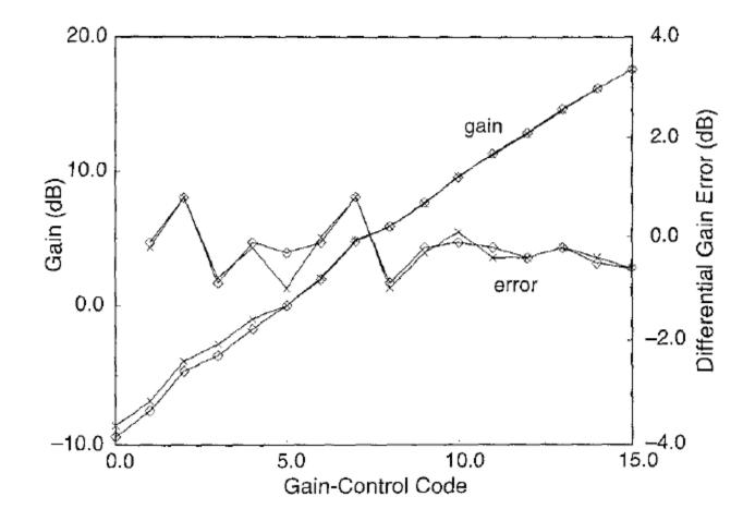
Figure 4: Amplifier gain and gain error.
