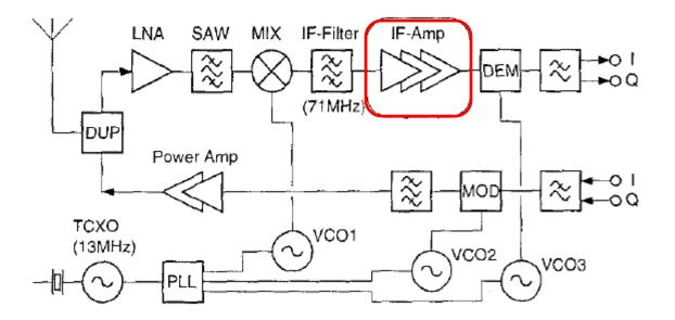
Figure 1: Block diagram of the GSM handset.
