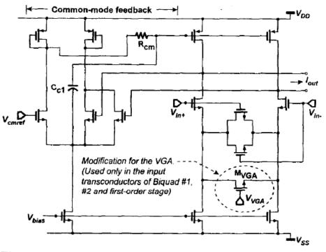
Figure 23.2.3: Complete transconductor.
