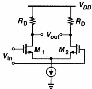
$$I_{D1} - I_{D2} = \mu C_{ox} \frac{W}{L} V_{OV} v_i \sqrt{1 - \frac{v_i^2}{4V_{OV}^2}} = \mu C_{ox} \frac{W}{L} V_{OV} v_i \sqrt{1 - x}$$
