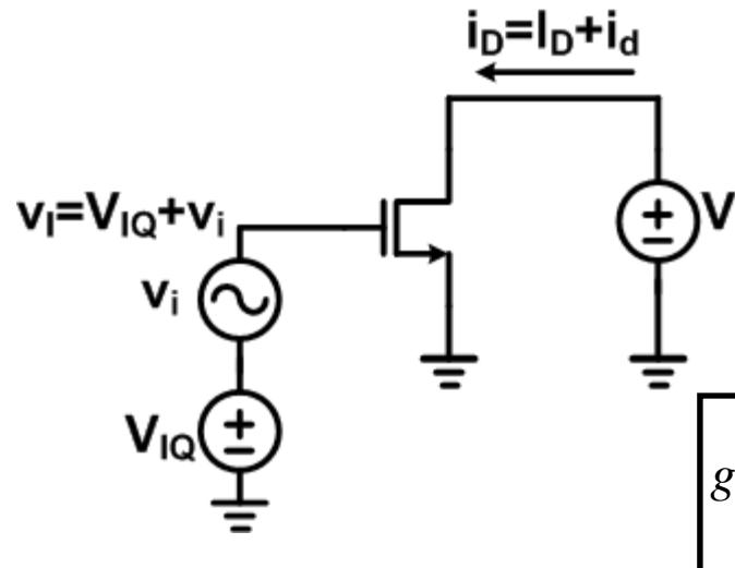
$$g_m = \left. \frac{\partial I_D}{\partial V_I} \right|_{V_I = V_{IQ}} = f'(V_{IQ})$$
