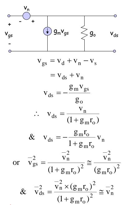
So for a diode the 1/f noise shows up as a noise voltage (shrinking the diode) of value equal to  $\overline{v}_n^2$ .
