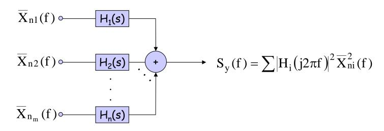
$\overline{x}_{n1}(f)$ ,  $\overline{x}_{n2}(f)$ , ... are uncorrelated noise sources
