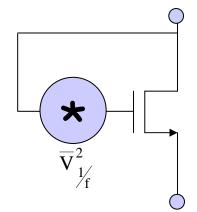
The noise can be seen as a drain-source noise voltage source equal to  $v^2_{1/f}$  (see next page)
