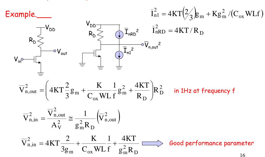
Can we always use the input-referred noise by a single voltage source in series with the input?
