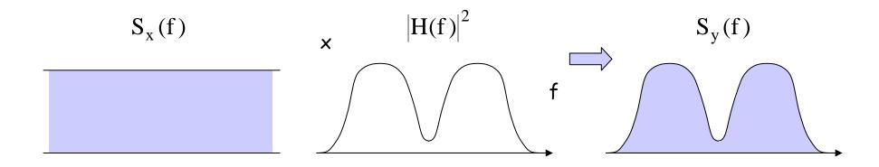
• A practical example is the telephone bandwidth, where BW of  $S_{\text{xin}}(f)$  is between 0-20KHz, BW of H(f) is 4KHz and consequently BW of  $S_{\text{yout}}(f)$  is 4 KHz.
