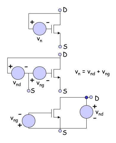
$$v_{nd} = g_m r_o v_{ng}$$
