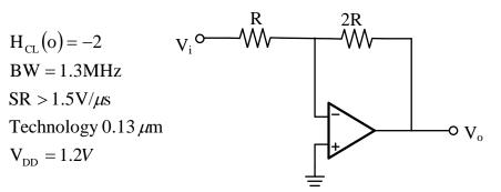
The accuracy error of the DC gain of the inverter should be less than 1.1%
