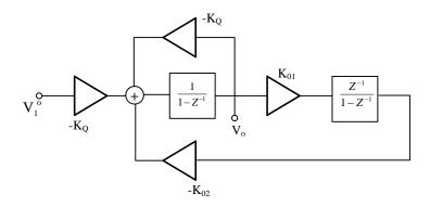
Using MATLAB (SIMULINK) or CADENCE macromodel simulate the filter shown above for r = 0.9710303 and  $\Theta = 35.957^{\circ}$
