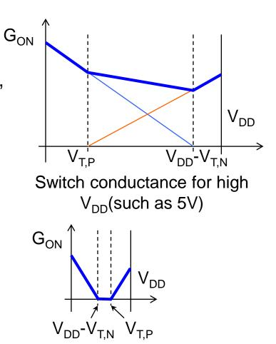
Switch conductance for low V<sub>DD</sub>
