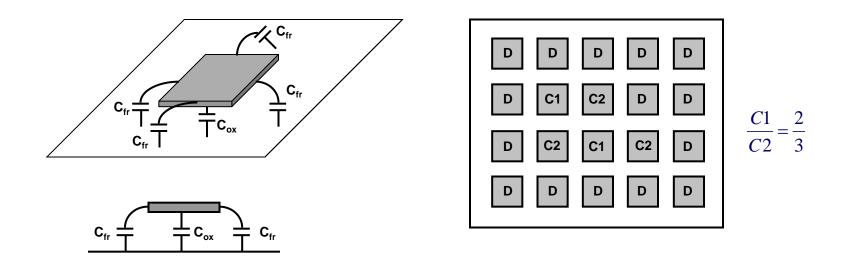
o Capacitor is implemented with PIP (poly) or MIM (metal)
