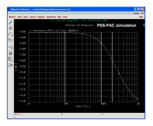
o PSS simulation is used to check the frequency response for Switched-capacitor circuito Should be compared with transient simulation
