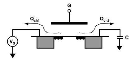
o During TR. is turned on, Q<sub>ch</sub> is formed at channel surface
