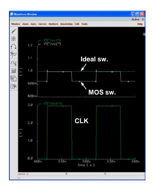
o When clock changes from high to low, Q<sub>ch2</sub> is injected to C
