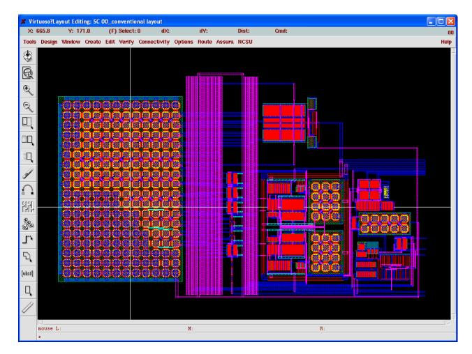
o Example of SC biquad circuit (TSMC 0.35um)
