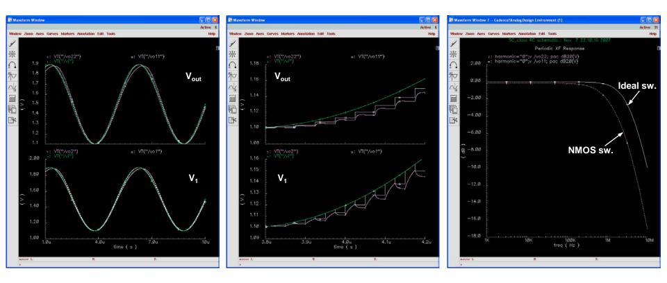
o Small NMOS sw. (5/0.4) o With high R<sub>on</sub>, output is not settled o In case of large signal input, N/PMOS sw. should be used
