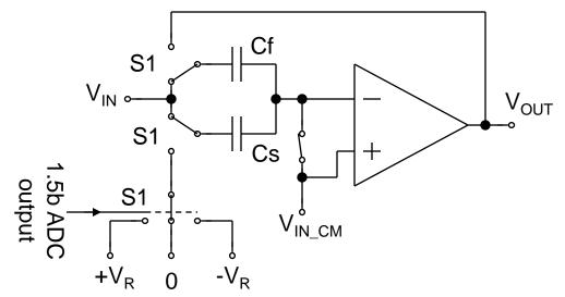
The X2 residue amplifier for 1.5b/stage pipeline A/D converter
