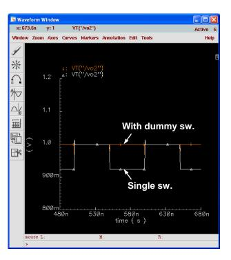
o Use dummy switch which provides opposite charge
