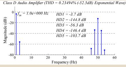
Class D output spectrum (SIMULINK simulation)
