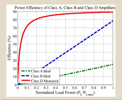
Continuously switch the output from one rail to another at supersonic frequency (Pulse Width Modulation -PWM-)
