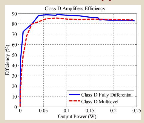
Class D fully-differential and multilevel have similar efficiencies and linearity but multilevel modulation gives better SNR and PSRR due to the extra level of quantization.
