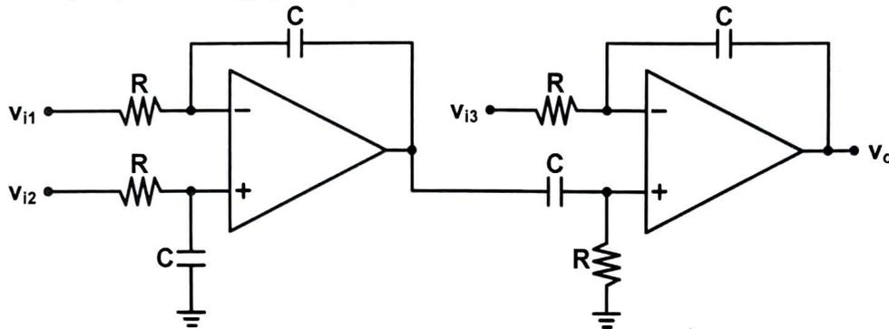
$$V_o = - \left( \frac{Z_c}{Z_R} \right) \left( \frac{Z_R}{Z_R + Z_c} \right) \left( 1 + \frac{Z_c}{Z_R} \right) V_{i1}$$
