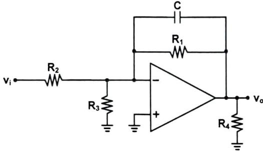
$$\frac{V_o}{V_i} = \frac{-Z_{R1} \parallel Z_C}{Z_{R2}} = -\frac{1}{\left(\frac{1}{R_1} + sC\right)R_2} = \frac{-\frac{R_1}{R_2}}{1 + sR_1C}$$
