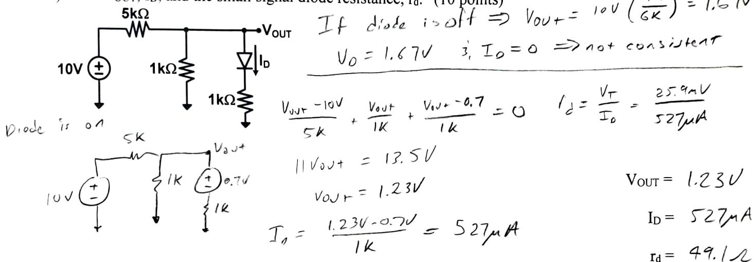
Assume for the following circuit that the diode is forward biased and there is a small-signal AC signal,  $v_{i,AC}$ , in series with a DC voltage.
