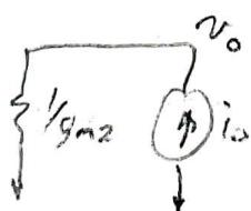
$$R_{out} = \frac{1}{g_{m2}} = \frac{1}{1.55mA/V} = 645\Omega \quad R_{out} = 645\Omega$$
