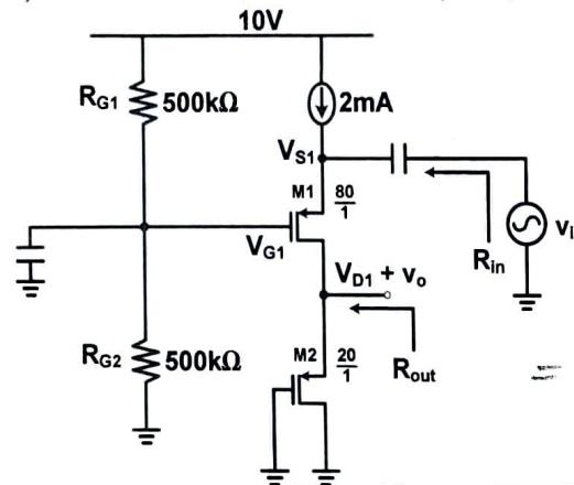
$$V_{D1} = \sqrt{\frac{2I_0}{K_P \frac{W}{L}}} + |V_{TP}| = \sqrt{\frac{2(2mA)}{30\mu(20)}} + 1V = 3.58V$$
