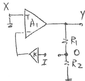
$$O = Y \frac{R_2}{R_1 + R_2} = (-IK)A_1 \left( \frac{R_2}{R_1 + R_2} \right)$$
