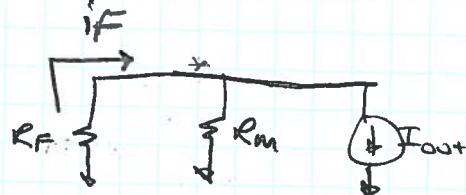
$$A_{I,CL} = \frac{g_{m2} (R_C \parallel r_{\pi 2})}{1 + \left( \frac{R_M}{R_F + R_M} \right) g_{m2} (R_C \parallel r_{\pi 2})}$$
