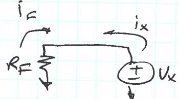
$$R_{in,OL} = R_F || r_{e1} \approx \frac{1}{g_{m1}}$$
