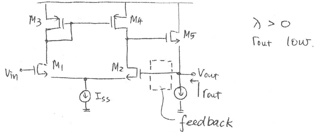
Note that  $V_{out}$  is directly fed back to input:
