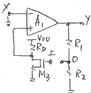
$$O = Y \left( \frac{R_2}{R_1 + R_2} \right)$$
