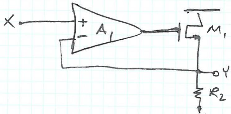
$$A_{OL} = \frac{A_1 R_2}{g_m + R_2} = \frac{A_1 g_m R_2}{1 + g_m R_2}$$
