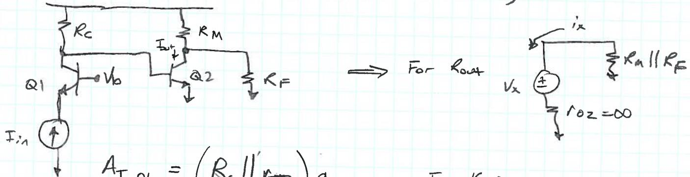
$$A_{I,OL} = \left( R_C \parallel r_{\pi 2} \right) g_{m2}$$
