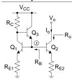
$$I_{o} \approx \frac{V_{CC} - 1.4}{R_{C} + R_{E1}} \frac{R_{E1}}{R_{E2}}, \quad V_{o,min} = V_{CE2,sat} + I_{o}R_{E2}$$
