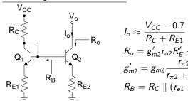
$$I_{o} \approx \frac{V_{CC} - 0.7}{R_{C} + R_{E1}} \frac{R_{E1}}{R_{E2}}, \quad V_{o,min} = V_{CE2,sat} + I_{o}R_{E2}$$
