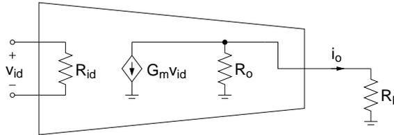
Figure 3: Equivalent small-signal model of the OTA.
