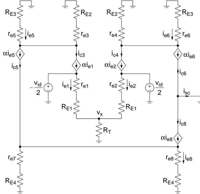
Figure 2: Small-signal circuit of the OTA.
