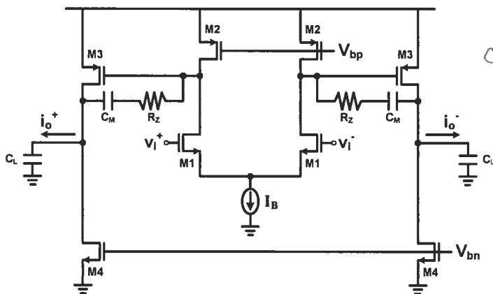
$$a. G_m = \frac{i_o^+}{v_i^+} = \left( \frac{-g_{m1}}{g_{o1} + g_{o2}} \right) (-g_{m3})$$
