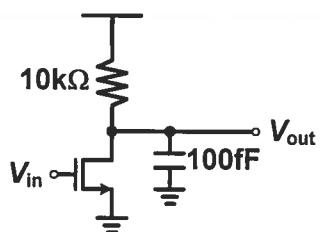
$$A_{DC} = -g_m R_o = -(1 \frac{\text{mA}}{\text{V}})(10\text{k}\Omega) = -10 \frac{\text{V}}{\text{V}}$$
