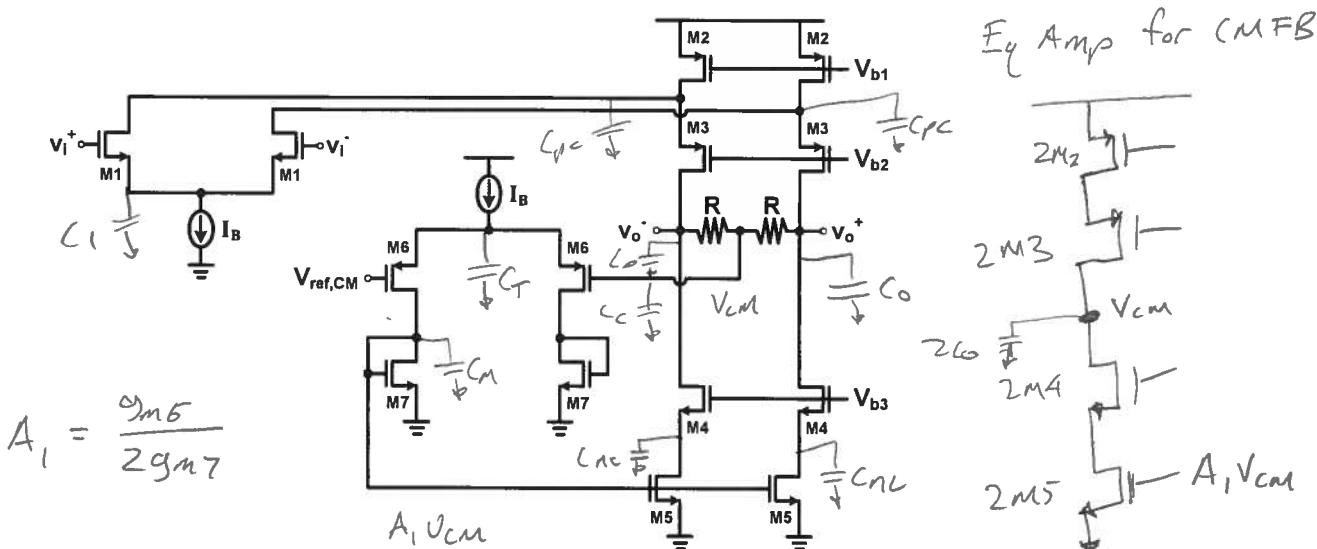
a.  $A_{vd} \cong g_{m1} \left[ g_{m3} r_{o3} (r_{o2} || r_{o1}) || g_{m4} r_{o4} r_{o5} \right]$
