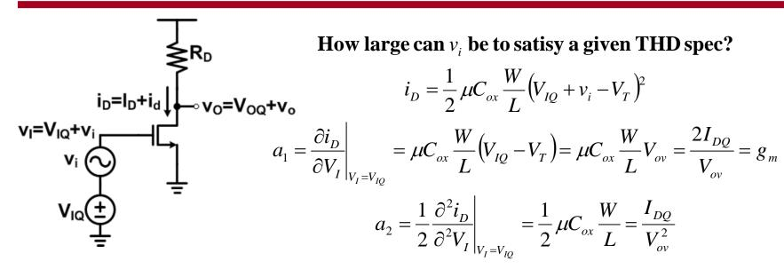
$$a_3 = \frac{1}{6} \frac{\partial^3 i_D}{\partial^3 V_I} \bigg|_{V_I = V_{IO}} = 0$$
