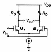
$$I_{D1} - I_{D2} = \mu C_{ox} \frac{W}{L} V_{OV} v_i \sqrt{1 - \frac{v_i^2}{4V_{OV}^2}} = \mu C_{ox} \frac{W}{L} V_{OV} v_i \sqrt{1 - x}$$
