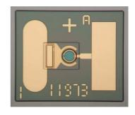
The APD can be operated at a low bias voltage of typically 29 V and has an excellent gain-bandwidth product of 90 GHz. The pad metallization is optimized for wire-bonding with the pads positioned to enable easy and direct bonding to most common TIA layouts. In addition, the small chip footprint saves valuable space in small packages such as TO-46.
