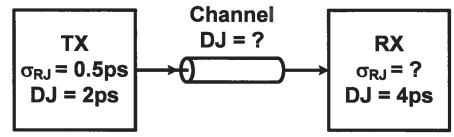
a) Assuming Gaussian pulse inputs, the SMF channel's DJ can be modeled as the difference between the output pulse width and the ideal 56Gb/s pulse width. What is the channel's DJ?
