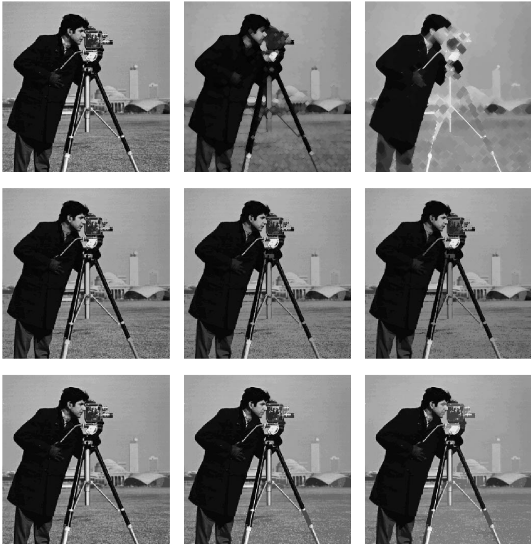
Figure 4: Illustration of scale-space representation. Top row: original grayscale image and markers. Middle row: evolution of the anti-extensive \sigma -reconstructive scale-space. Bottom row: evolution of the extensive dual \sigma -reconstructive scale-space.
